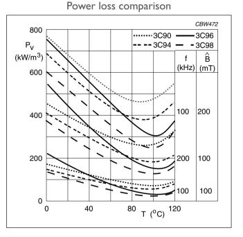
Together with FXC 3C90 and 3C94 completes the low loss power conversion material family with optimal working temperature at 100°C.
